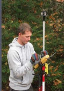
Jeff using the data logger with the new Robotic Total Station. The mirrors at the top of the rod reflect the total station's laser back to the unit in order to accurately measure distance.
