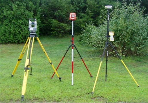
The primary data collection devices used during the internship. The Total Station pictured here (left) has been replaced by a Robotic Total Station that can be operated by a single user. At center is the reflecting rod used with the total station. At right is the RTK GPS unit. The 'bell' on top is the receiver and the removable handheld device located mid-shaft is the data logger that allows the user to store information about the points collected.
