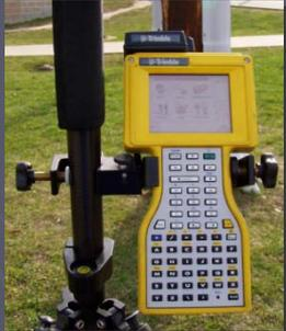
The data logger used with the RTK GPS unit. Users document feature attributes using attribute libraries which are designed prior to entering the field.
