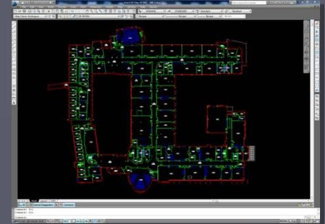
This CAD drawing represents the starting input that the model extracts data from. Individual room lines were ultimately converted to polygons according to the operations built into the model.
