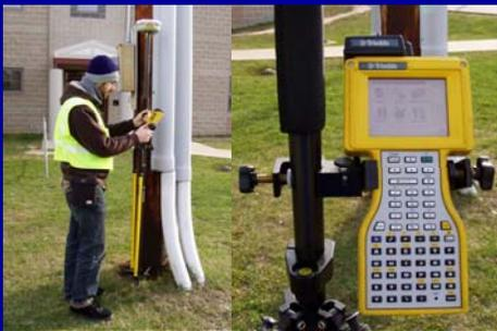
The RTK GPS unit was used to measure the precise location of utility poles and store that information in the Trimble data logger via Bluetooth. Trimble Geomatics Office was then used to check the data into ArcMap.
