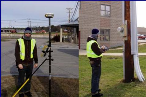
These two photographs show Joe measuring an offset point with the RTK GPS unit and collecting utility pole attributes with the tablet PC.
