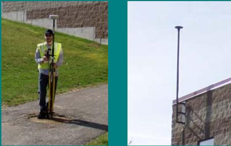
These photographs show Guerra measuring the location of a sewer manhole with the RTK GPS unit. The RTK GPS unit connects to the UNH Base Station to find sub-centimeter accuracy.
