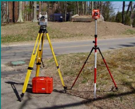
The Total Station and Reflecting Rod were used to survey manholes that could not be collected with the RTK GPS unit. The Total Station required a two-man team and was more time consuming.
